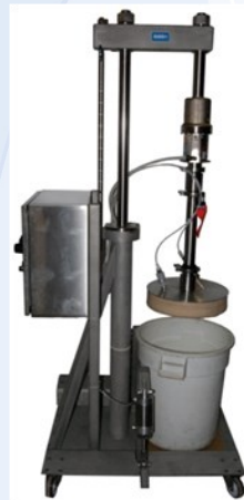
Portable sanitary single post ram with mechanical safety stop and pneumatic control box
