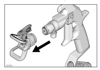
3. Unscrew cap, remove filter. Assemble without filter. Clean filter.
