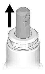
2. Push pin (31) into hole. Push retaining ring spring into groove all the way around connecting rod.
