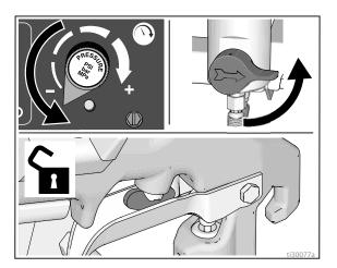
Hold gun against grounded metal flushing pail. Trigger gun and increase fluid pressure slowly until pump runs smoothly.
