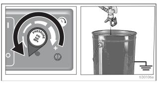
4. Engage the trigger lock. Turn prime valve down.
