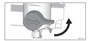
8. Hold gun against paint pail. Disengage gun trigger lock.
