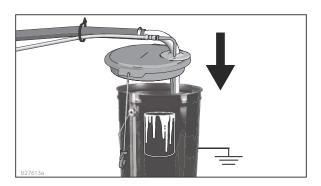
12. Trigger gun again into flushing fluid pail until paint appears. Assemble Rac Tip and Rac Guard.
