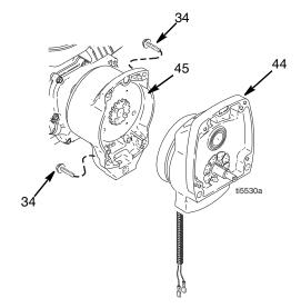
5. Place pinion assembly (44) on bench with rotor side up.
