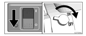
3. Turn pressure to lowest setting. Trigger gun to relieve pressure.
