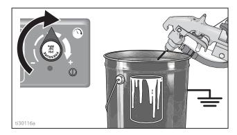
10. Move gun to flushing pail, hold gun against pail, trigger gun to thoroughly flush system. Release trigger and engage trigger lock.
