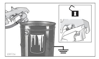
9. Gradually turn pressure control up until motor begins to drive pump. Trigger gun until flushing fluid appears.
