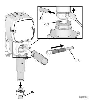
5. Loosen jam nut by hitting firmly with a hammer. Unscrew pump.
