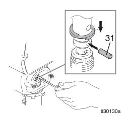
3. Screw jam nut down onto pump until nut stops. Screw pump up into drive housing until top threads of pump are flush with drive housing face. Back off pump and jam nut to align pump outlet to side. Tighten jam nut by hand, then tap 1/8 to 1/4 turn with a 20 oz (maximum) hammer to approximately 75 ±5 ft-lb (102 N·m). Connect hose (118) and suction hose (57).
