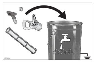
Remove siphon tube set from paint and place in flushing fluid. Use water or pump conditioner for water-base paint and mineral spirits for oil-base paint.
