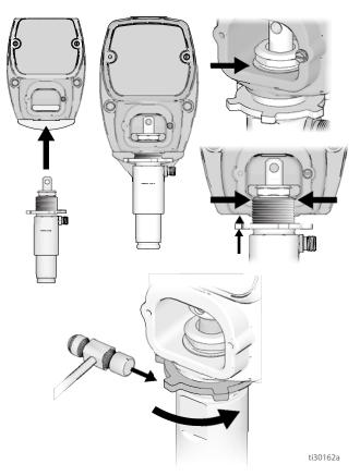
4. Fill packing nut with TSL until fluid flows onto the top of seal. Install pump rod cover (107).
