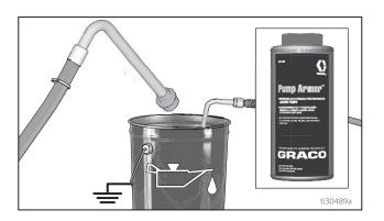
14. Close prime valve. Trigger gun into flushing pail to purge fluid from hose. Open prime valve.
