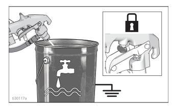
11. Open prime valve and allow flushing fluid to circulate for 20 seconds to clean drain tube.
