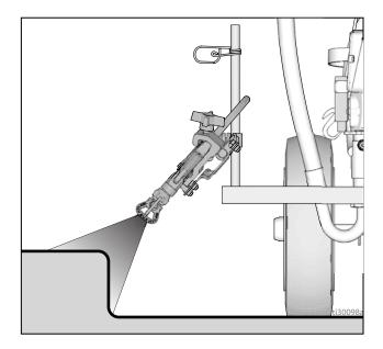
5. For **Gun Arc Spray Position**, place gun at rear of striper. Rear position improves arc quality.
