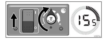
Turn pressure down, close prime valve. Disengage gun trigger lock.
