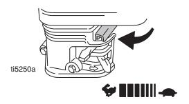
d. Set engine switch to ON.
