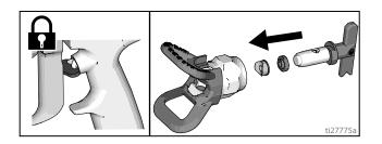
3. Screw assembly onto gun. Hand tighten.
