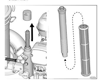
4. Clean gun filter, Rac Guard and Rac Tip in flushing fluid. See **Flushing Recommendations**, page 21.
