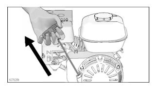
f. After engine starts, move choke to open.
