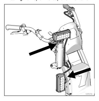
4. Route wires up to the battery and connect to the (+) and (-) terminals.
