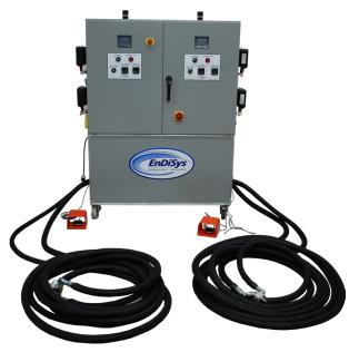
In one application, a material supplier needed a high flow, wide ratio machine to inject an atmospheric activating curing agent into silicone during the manufacturing process. EnDiSys designed a 30 GPM 160:1 ratio machine and a special static mix assembly to meet the customer's needs.
